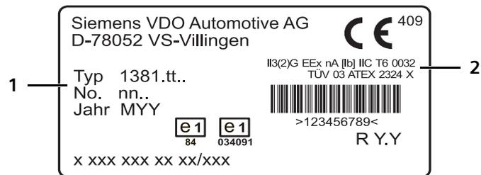
Fig. 6 - 3: Model plate DTCO 1381 (ADR variant)
